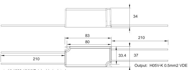
Input: UL1332 18AWG / double isolated
